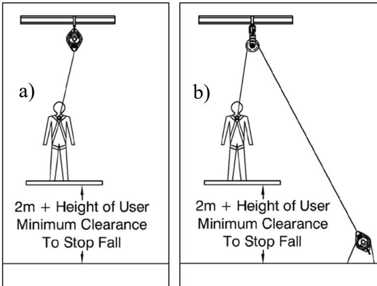
The anchorage for the G.Saver II should be positioned so as to:
