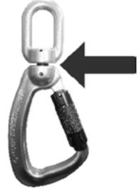
Check the safety hook and its gate locking function, and that the fall indicator has not activated (if present). If activated, the pin that connects the swivel eye and the hook (highlighted in the image by the arrow) will show red.
